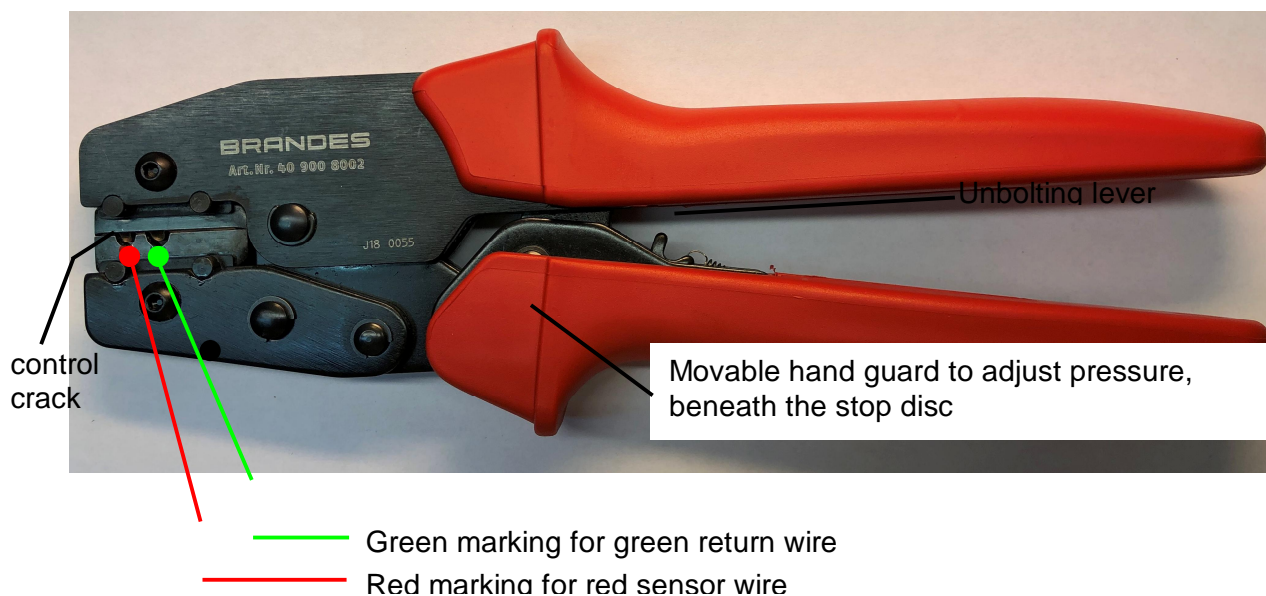
Fig. 12.1 Crimping plier BS-QZ22
